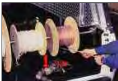
Quick Spool & Reel Holder Sets up in seconds, insures wire unspools correctly and allows multiple wires to be pulled off simultaneously (1" pipe not supplied.) Stainless steel.
