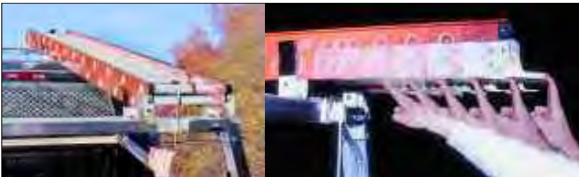
Ladder Roller and Clamp System Provides near effortless loading, unloading, and fastening of a single ladder. Ladder rolls forward to front hold-down and is clamped in rear with one motion. Typical ladder lengths are 24' and 28'. Call for info on your particular application. Aluminum and stainless steel with ultra high molecular weight polyethylene rollers.
