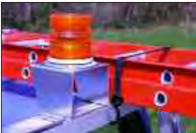
Strobe/Antenna Mount, high profile 6" tall for protection from ladders, 3/4" center hole, 3 oblong holes 120° apart for strobe mounting bolts. Aluminum.
